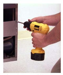
Removing gas manifold shield.
